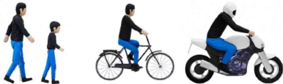
Figure 5-1: Euro NCAP VRU Targets (EPTa, EPTc, EBT and EMT)
